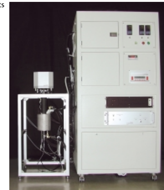
Apparatus for the combined volumetric-gravimetric measurement of co-adsorption equilibria of binary mixtures. Development made in co-operation between Rubotherm and BEL Japan Inc.
