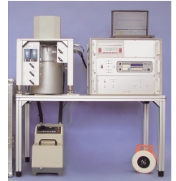
Portable densitometer to calibrate vibrating gas density transducers in natural gas pipelines, Chair of Thermodynamics, University of Bochum
