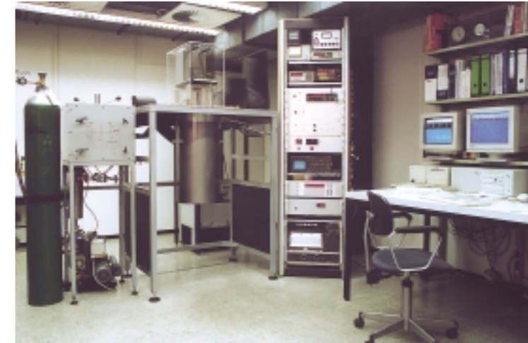
Apparatus for the simultaneous measurement of viscosity and density at the Chair of Thermodynamics at the University of Bochum
